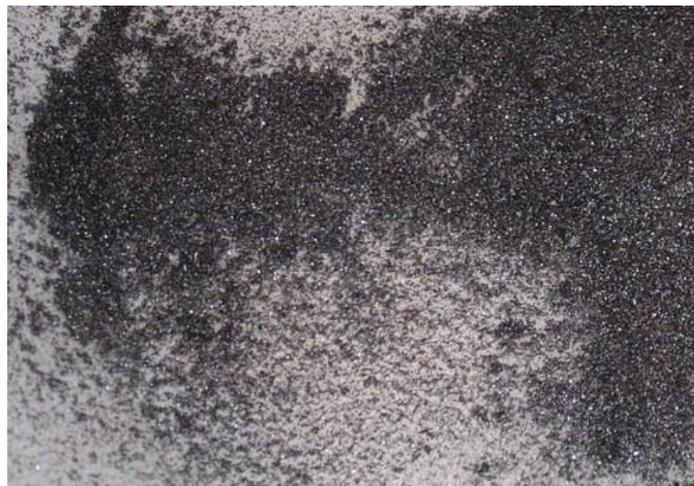
Figure 2: Functionalized MWCNTs powders exhibiting lustrous appearance
