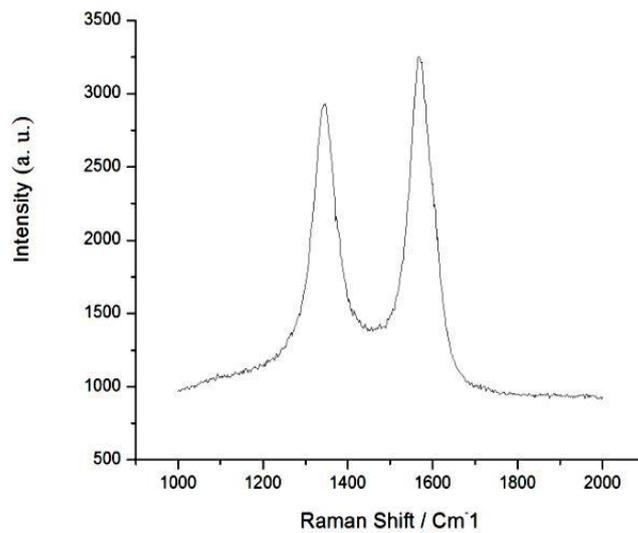
Figure 1: Raman Spectra of Multi-Walled Carbon Nanotubes
