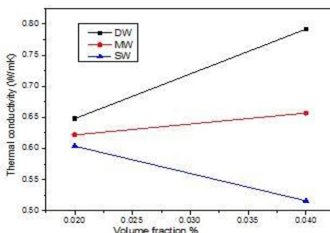
**Figure 4: Variation of Thermal conductivity of Different Water Samples with Varying Volume Fraction of MWCNTs**
